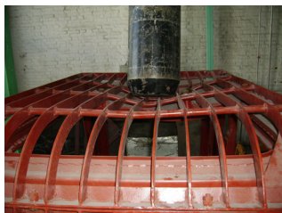
Figure 6. Experimental residual deformation of top guard
