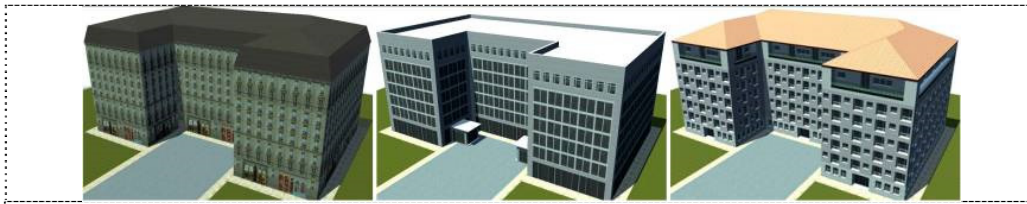
Figure 3. Automatically generated façades based on procedural modeling
