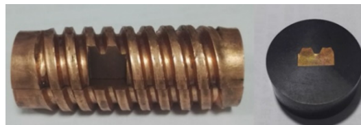
Figure 11. Metallographic specimen of tooth
