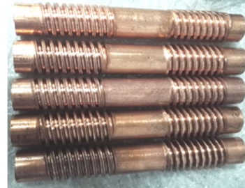
Figure 3. Rolling forming process of worm Figure 4. Worm experimental part
