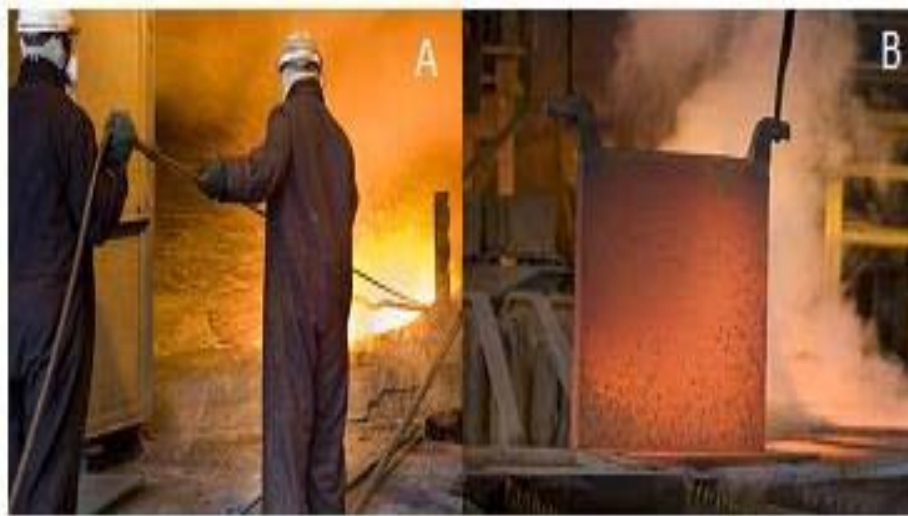
Figure 2: Images of (A) PC's existing reverberatory furnace and (B) off-gas from the reverberatory furnace [6].
