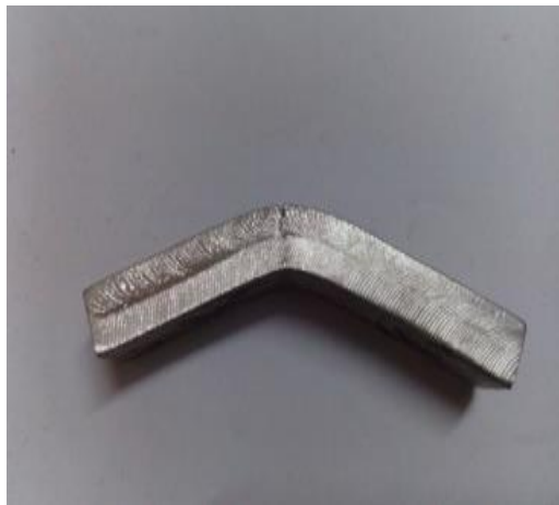
Figure 4. Flexure sample after testing.
