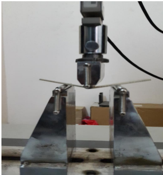
Figure 2. Flexural Test Specimen loaded in a three point flexure attachment
