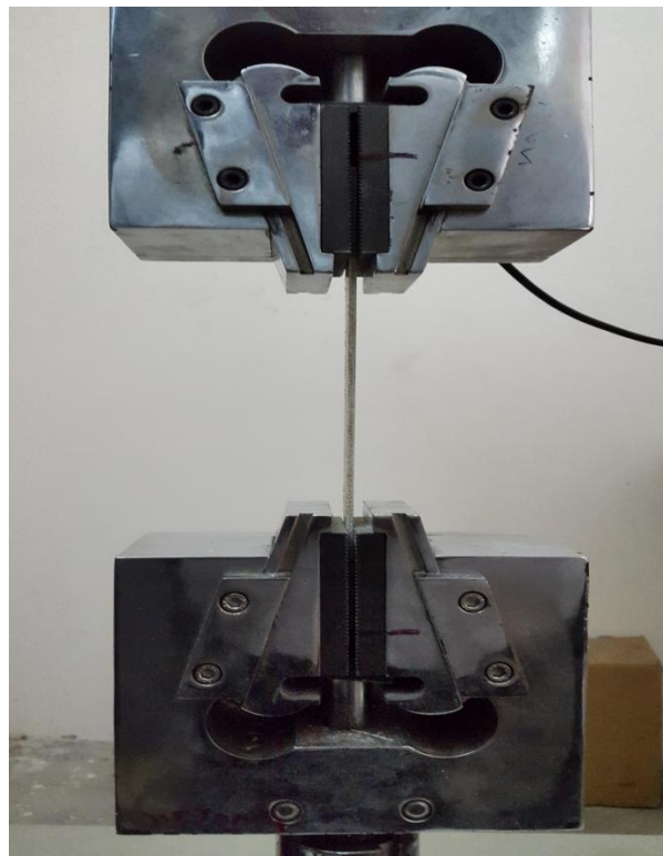
Figure 1. Tensile test specimen loaded in the UTM
