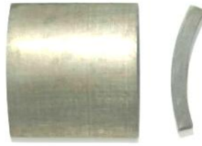
Figure 1 Photographic view of cylinder liner and piston ring segment
