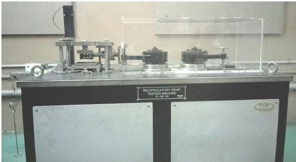
Figure 2 Photographic view of HFRR tribometer
