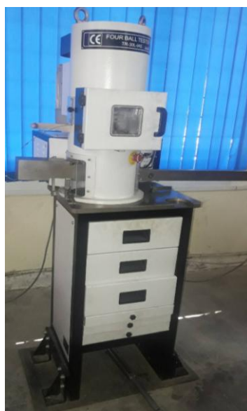
Figure 1 Four ball wear tester
