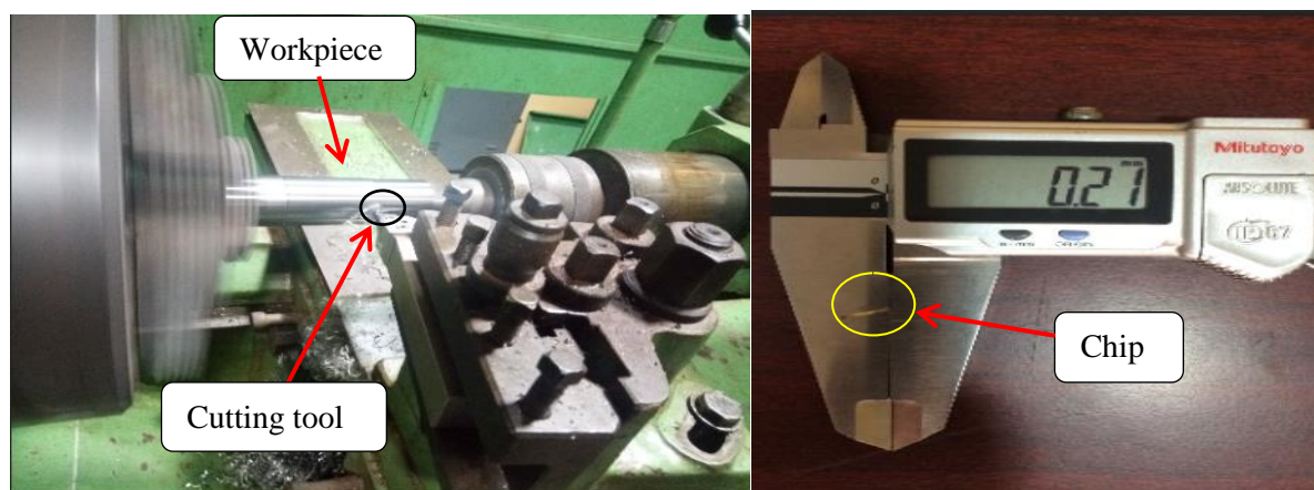
Figure 1. (a) Experimental set up (b) Chip thickness measuring instrument (Digital Vernier calliper)
