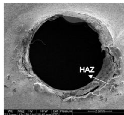
p. Laser drilled hole at exit at 3200 Watt, 4 bars using N 2
