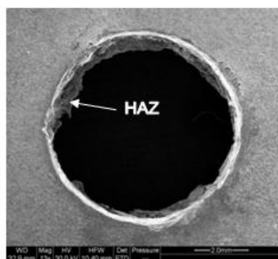
o. Laser drilled hole at entry at 3200 Watt, 4 bars using N 2
