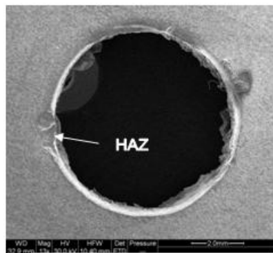
m. Laser drilled hole at entry at 3200 Watt, 5 bars using N 2
