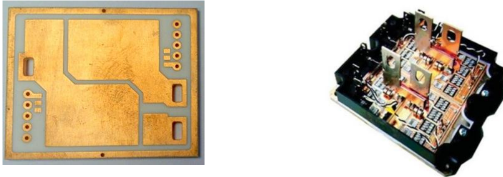
Figure 1. Typical commutation board and view of the power electronics module.
