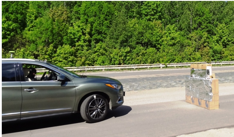
Figure 1. The maneuver around an obstacle (soft wall)
