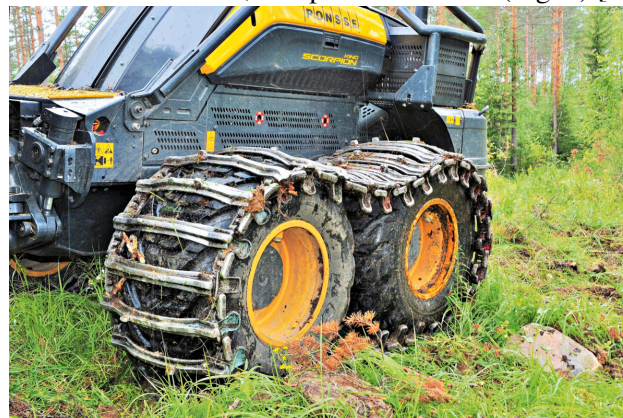
Figure 3. Standard bogie track sagging
