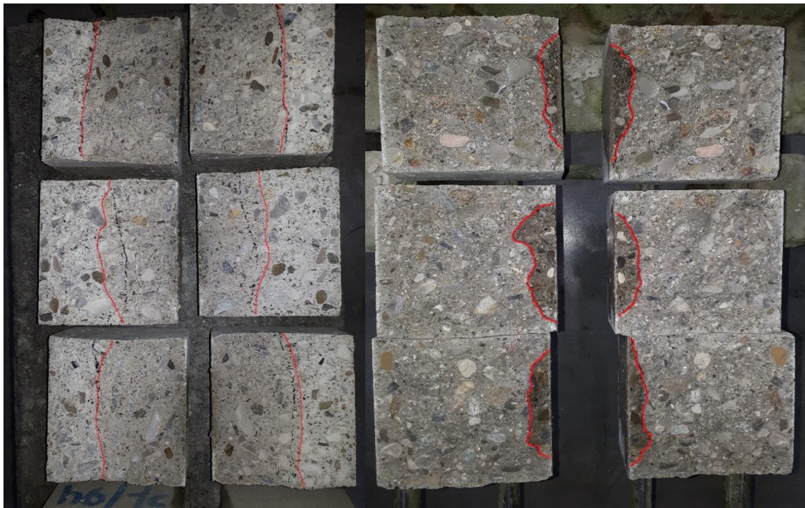
Figure 3. Split samples after water penetration test, red line marks the maximum depth of water penetration, samples treated by COMP procedure are on the left, and samples treated by REF procedure are on the right.
