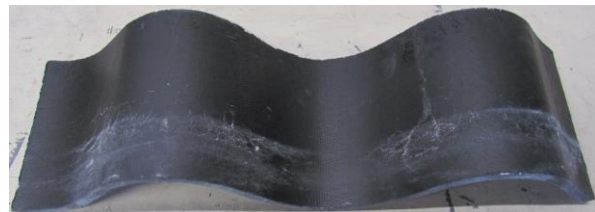
Figure 3. Sample of fibre-cement profiled sheet after 100 cycles of freeze-thaw.
