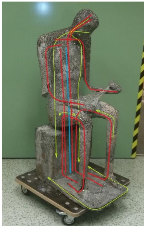
Figure 7. The anticipated pathways of the detected reinforcement in the sculpture. Red – rectangular cross-section of 10 x 10 mm, green – circular cross-section of Ø 6 mm, blue – reinforcement with an unknown cross-section with a width (diameter) of min. 15 mm. Reinforcement of the mandolin and fingers with reinforcing bars of Ø 6 mm is not captured in the picture.
