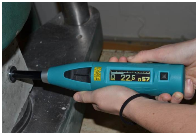
Figure 1. Test hammer SilverSchmidt PC L with the mushroom plunger [1].
