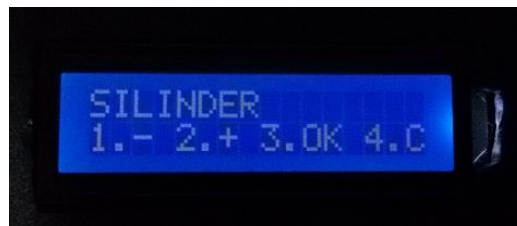
Figure 7. LCD display to select the container shape used.
