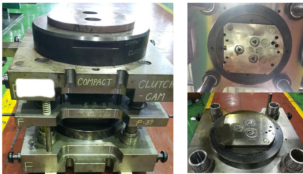
Figure 6. Fabricated compound fine blanking tool.
