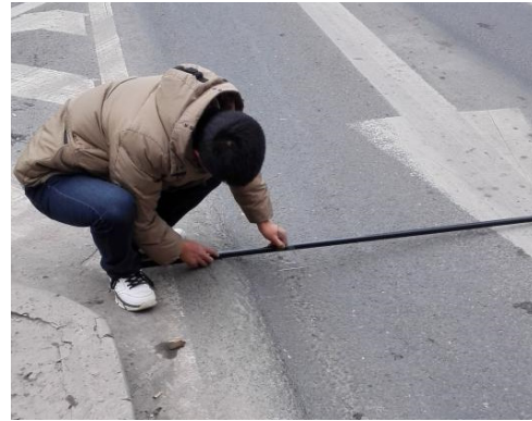
Figure 2. Intersection Rutting
