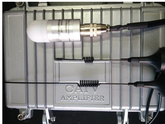
Figure1. MEMS Electric Field Measurement Device
