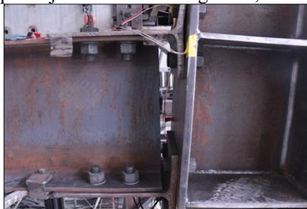
Figure 9. Fracture failures of plane joint.
