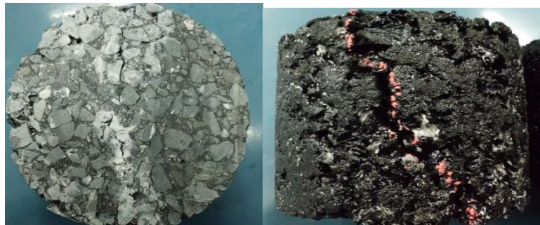
Figure 3 IDT sample and uniaxial sample failure state
