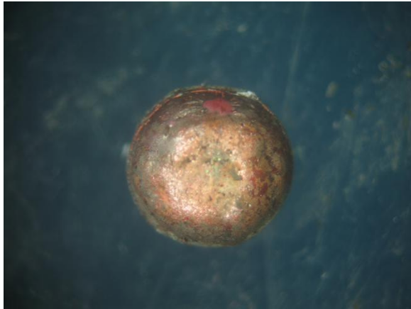
Figure 5 external appearance of a spark generated at 6I_e 8\times
