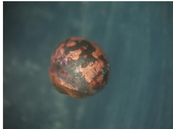
Figure 4 external appearance of a spark generated at 5.5I_e 8×
