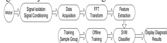
Figure 1. The hardware structure of the system
