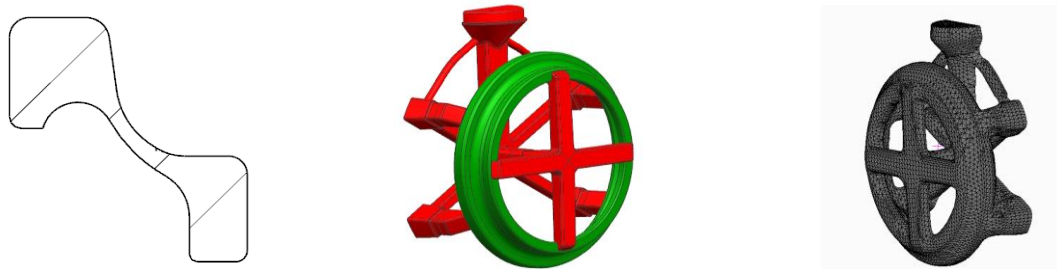
(a) Ring section (b) Geometry model of casting system (c) Grid model of casting system
