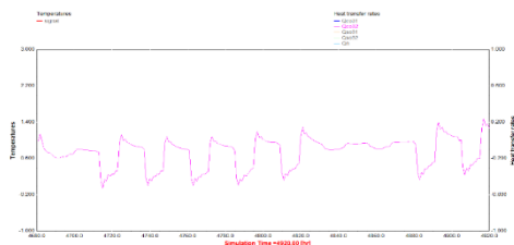
Figure 6. Heat exchange Q_{co, \text{floor}} of the floor with a PCM layer
