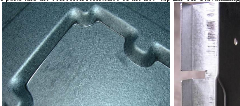
Fig. 1 The blackening phenomenon during the drawing process
