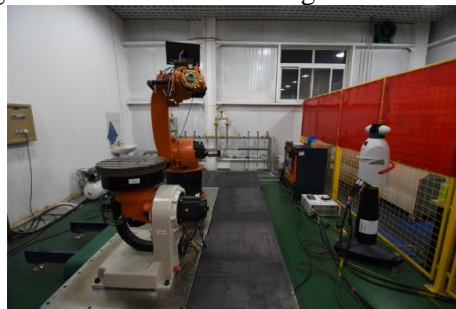
Figure 8 Using Laser Tracker to Measure the Standard Tool
