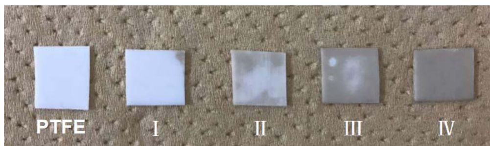
Figure 6. The morphologies of sonicated PDA coated PTFE. All the samples were sonicated for 90 min
