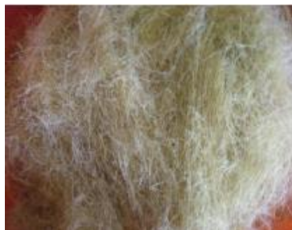
Figure 5. Bamboo fiber processed with untreated bamboo
