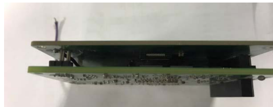
Figure 10. Sensor board and FPGA board structure
