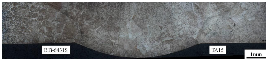
Figure 2. The profile of butt joint by TIG welding
