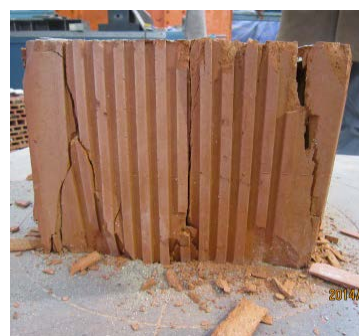
Figure 2. Failure form of the block
