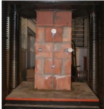
Figure 4. Layout of dial gauge
