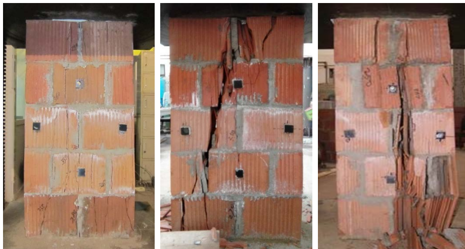
Figure 6. Failure modes of prisms
