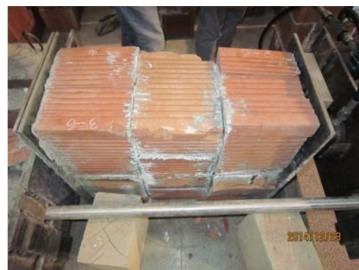
(b) Shear compression failure
