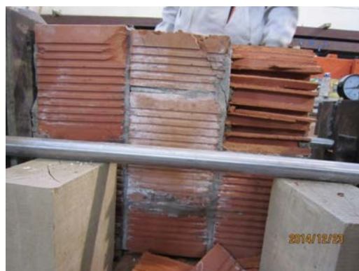
(c) Local compressing failure
