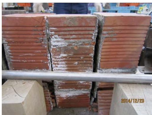
(a) Shear friction failure
