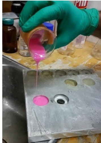
Figure 1. Casting of silicone rubber (Elite double 8) after vigorous mixing.
