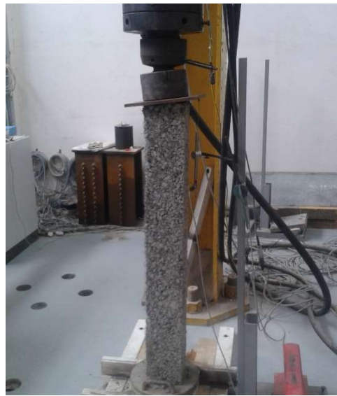
Figure 4. Specimens after laboratory tests 150/150/1,200 mm.
