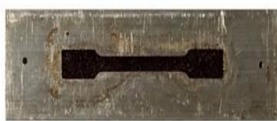
Fig. 2, 3 and 4 metallic mould for specimen, mould with specimen and ejected specimen
