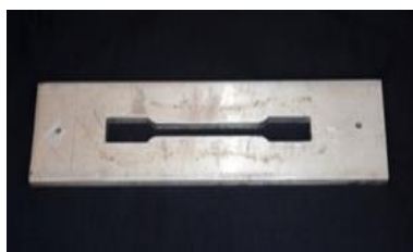
Fig. 2, 3 and 4 metallic mould for specimen, mould with specimen and ejected specimen
