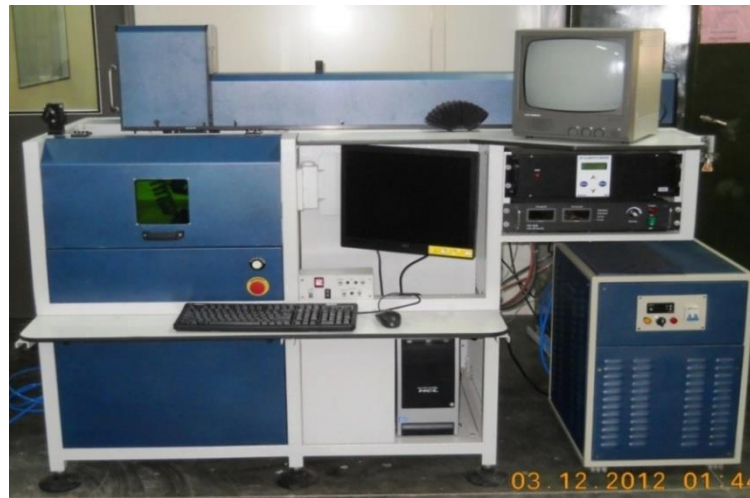
Figure2.2 Photographic view of diode Nd: YAG laser machining system
