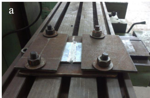
Fig. 1(a) Fixture developed for FSW process (b) Tools with different pin arrangements used for the experiment: (A) Triangular profile (B) Square profile (C) circular profile
