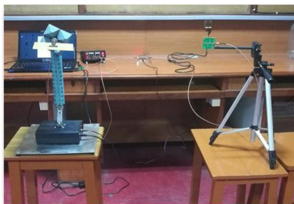
Figure 17. AMITECH Gain measurement set-up
