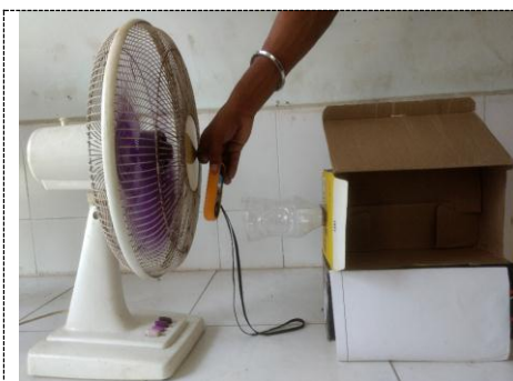
Figure 6. Measuring the velocity and temperature of air at the entry of specimen 1
