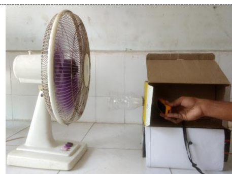
Figure 7. Measuring the velocity and temperature of air at the exit of specimen 1
