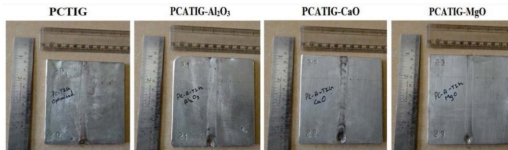
Figure 1: Welded samples of PCTIG, PCATIG- \text{Al}_2\text{O}_3 , PCATIG- \text{CaO} and PCATIG- \text{MgO}
