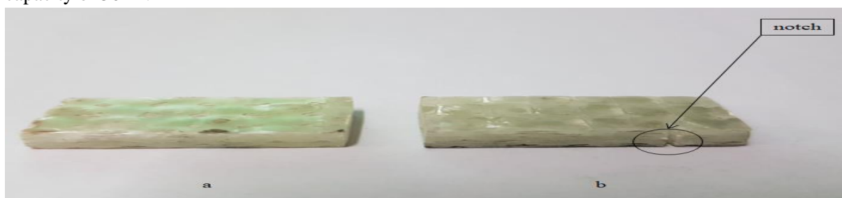
Figure 2. Sample laminates of neat laminate composite for Short Beam Shear Test (a) without pre-crack (b) with pre-crack.
