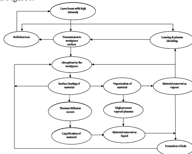
Figure 1. Block diagram of laser micro drilling showing mechanical mechanism
