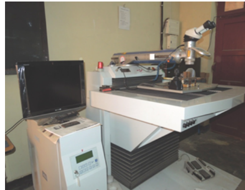
Figure 3. CNC pulsed Nd:YAG laser M/C system
