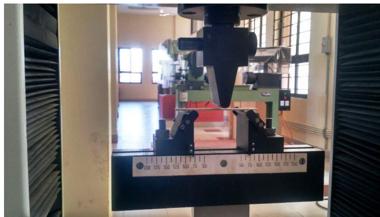
Fig. 4 Flexural test setup
