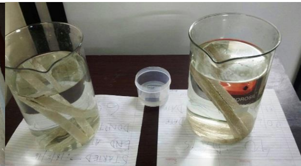
Fig. 2 Ageing of composite specimens
