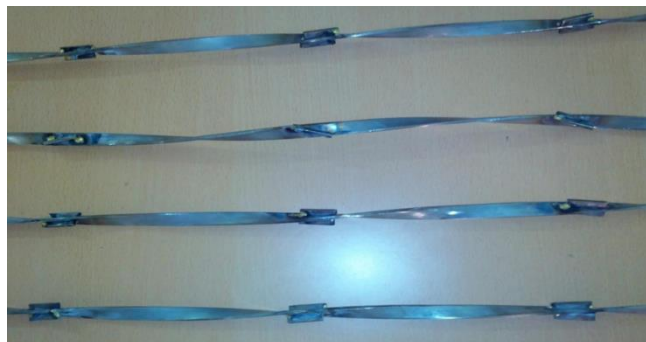
Figure 3: Baffled twisted tapes of width 12mm, twist ratio 2.2 and length 825mm
