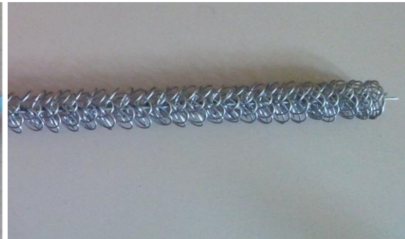
Figure 5: hiTrain wire matrix with 14 mm outer diameter, 1.2-1.6mm centre wire diameter, 190-210 loops per foot and length 825mm
