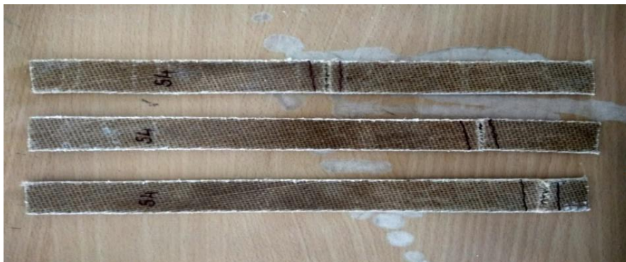
Figure 5: JS4 Tensile Specimen Failure Pattern
