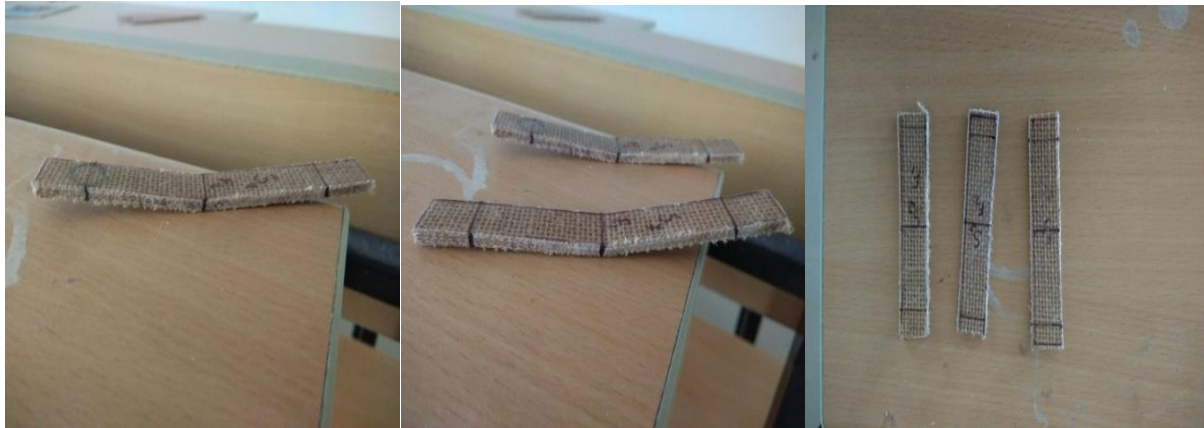
Figure 16: JS4, JS7, FS2 Flexure Specimen Failure Pattern
