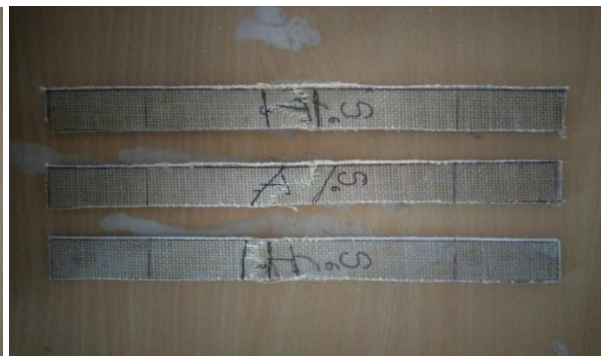
Figure 10: JS6 Tensile Specimen Failure Pattern
