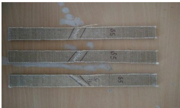
Figure 9: JS5 Tensile Specimen Failure Pattern
