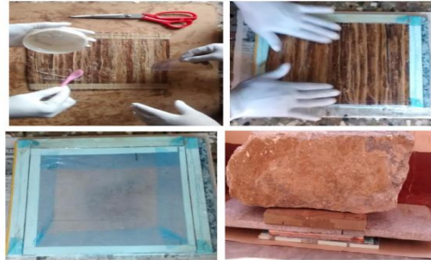
Figure 2 Hand layup technique
