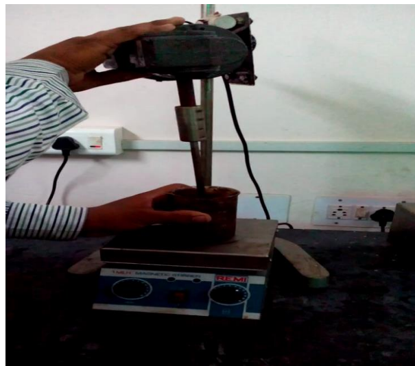
Figure 1. Illustrates mixing of the epoxy resin, coconut shell powder, and hardener
