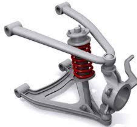
Figure 2- Double Wishbone Suspension System
